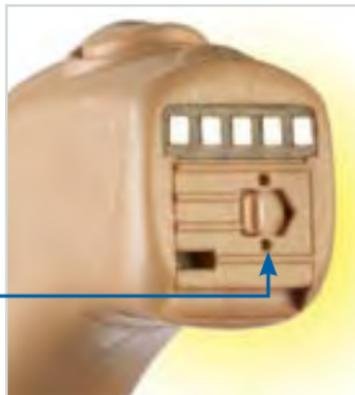
To lock the door, use an appropriate tool to slide the recessed switch to the left until it “clicks” and the colored mark is visible. Locking the door is **not** necessary for operation.
