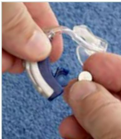
To insert or replace the battery, open the battery compartment by placing your fingernail under the edge of the swing-out door and gently pulling away from the instrument.
