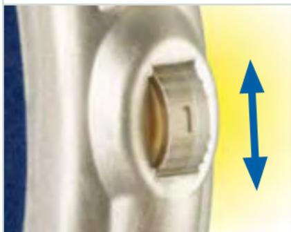
The volume control enables you to adjust the amount of amplification provided by the instrument. You may wish to change levels as you encounter
