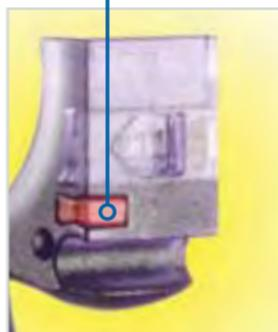
Your BTE uses a size 13 battery as its power source. This battery size can be identified by the orange color code on the packaging. Be sure to use the correct size and type cell for your instrument. Because of their size, it's a good idea to change and replace batteries above a table or desk to reduce the risk of dropping the instrument or battery.
