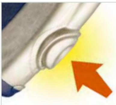
The telecoil is manually activated by pushing the control to access the memory containing the telecoil function.
